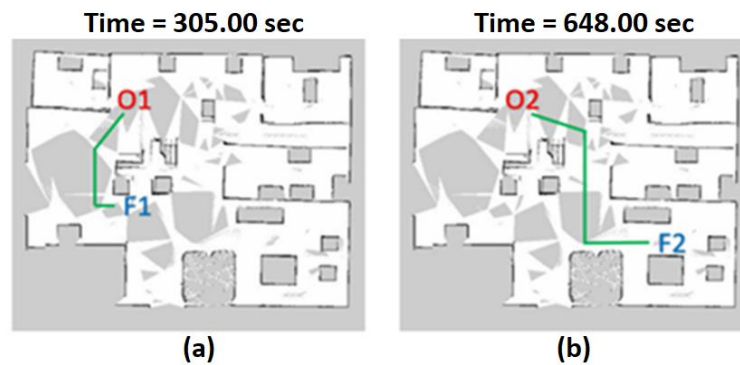
Figure 12. Example of the time for different paths. In this example, in the simple path (a), the robot requires less time to arrive to the target point in comparison with the complex path (b).
