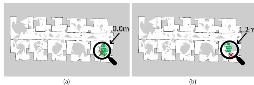
Figure 13. Examples of the mean error value for different paths. In this example, in the simple path (a), the distance between the robot and the target point is less than in the complex path (b).
